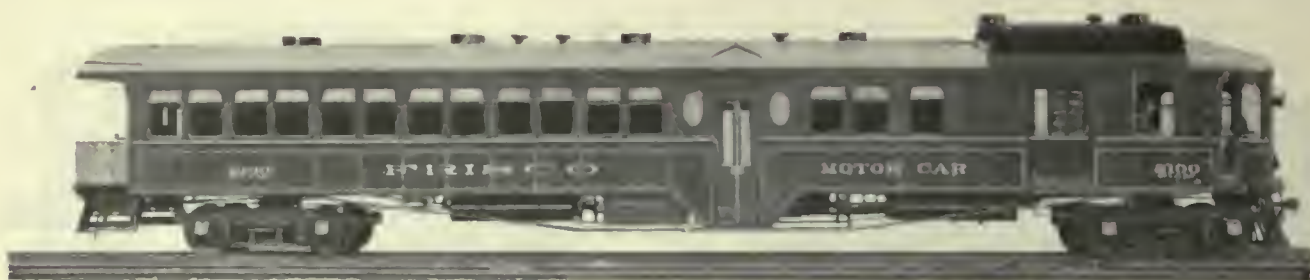
FIG. 439. TYPICAL GASOLINE-ELECTRIC CAR BUILT BY THE GENERAL ELECTRIC COMPANY
